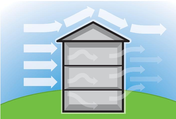
*Permeable insulations, such as cellulose and fiberglass, are more susceptible to air infiltration and air leakage than ccSPF insulation.*
